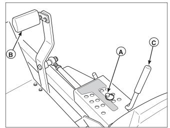
Figure 37. Mowing Height Adjustment A. Cutting Height Adjustment Pin B. Deck Lift Foot Pedal
